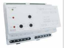
The synchro-check (paralleling) protector trip relay compares the voltage, frequency and phase angle of two supplies and operates a relay according to the state of synchronisation of the supplies. If the two supplies are not synchronised, the relay operates to provide a control output. The relay output can be used for alarm or control purposes.
