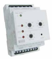
The Speed Sensing protector trip relay monitors rotating equipment using a magnetic pick-up and provides three output contacts which can be used to initiate alarms or shutdown signals. The relay also provides a tachometer output for speed indication.
