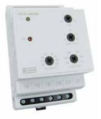
The phase balance, sequence and voltage protector trip relay, is designed to monitor a three-phase supply for phase imbalance, low or missing phases or incorrect phase sequence and to trip a relay if it detects any anomaly. Two versions are available to suit either three-phase three-wire (PSF/G3) or three-phase four-wire (PSF/G4) systems.
