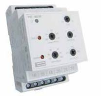
When the measured voltages moves outside the set point limit for longer than the time delay, the relay will operate giving an alarm control or tripping signal. The Protector can be used for under and over voltage detection, start standby generators, operation of mains failure units and switching standby suppliers. An illuminated red LED indicates a fault condition. The three-phase, three or four-wire models with protect each phase independently.
