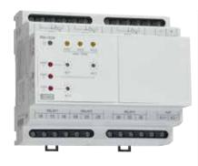
The hot spot 3 relay accepts up to three inputs from resistance temperature detectors (RTD) and provides up to three user adjustable trip points which can be used to initiate alarms, cooling system or shutdown. The relay is ideally suited for the protection of electric motor windings, transformers, generator winding and bearing temperature. The analogue output can be used for remote monitoring of high temperates.
