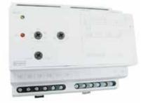
AC current protectors provide a continuous surveillance of monitored circuits and offer user adjustable trip points (set points) with time delay settings. When the current moves outside the set point limit for longer than the time delay, the relay will operate providing an alarm control or tripping signal.
